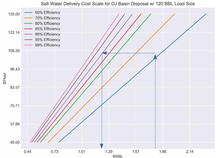
Fig. 1 – Saltwater delivery cost scales modeled using the Revonos Limitless Delivery Office Analytics module.
